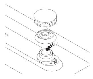
The presence of dirt inside the appliance can obstruct the nozzles, affecting the flame.
