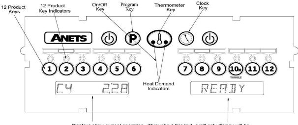
Displays show current operation. Throughout this text, a left only display will be printed as [C4 2:28]. When both left and right displays should be interpreted together, this text will show them as [C4 2:28] [READY].
