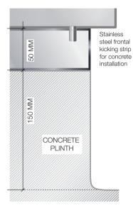
Accessories for installation on 150 mm high concrete plinth are available on request.
